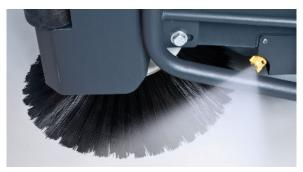
Patented DustGuard<sup>™</sup> is proven to reduce airborne dust generated by side broom sweeping. An ultra fine fog suppresses fugitive dust
