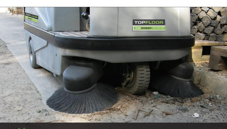
When sweeping floors with a mix of large debris and a high volume of dust, the TFIIOR-TRS comes out trumps every time.
