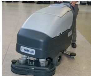
11. Push the drive paddle for starting floor cleaning. If solution applied flows outside the brush housing during use, reduce the flow of solution. Switch off the machine using the key.
