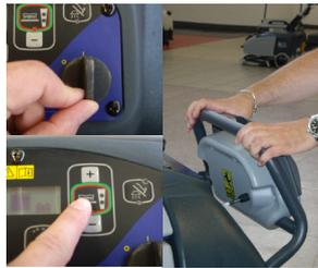
6. Turn the ignition key to "I", then lower the deck by pressing the Green switch. To engage the brushes, slightly press the drive paddle and then release it.
