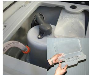
13. Wash with clean water the recovery tank and the vacuum grid. Remove and clean the debris tray.
