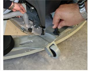
4. Install the squeegee and fasten it with the handwheels, then connect the vacuum hose to the squeegee.
