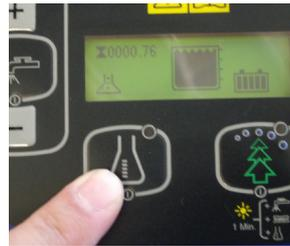
8. Press the detergent flow control switch. The number of display shows the detergent concentration level in the solution (see the table on the label). See the User Manual for setting change.
