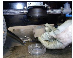
14. Clean the filter: 1) Close the solution tap under the machine. 2) Remove the transparent cover and the gasket, then remove the filter strainer.
