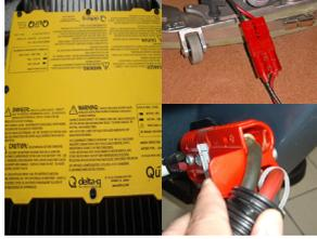
1a. Switch off charger by pressing the STOP button. Unplug charger cable from red battery plug. Reconnect the red battery plug to the machine.
