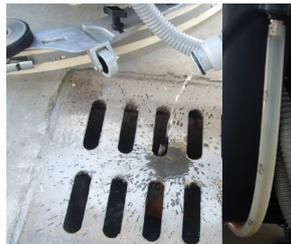
12. At the end of the work. Empty the recovery tank with the hose. Then empty the solution tank with the transparent hose
