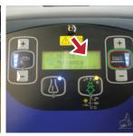
2 Check if there isn't any brush motor overload i.e. 3 battery Ledsflash simultaneously or error code on dis-
