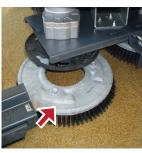
1 Check if the brushes are correctly installed and not worn out.
