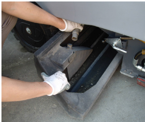
16. Remove and clean the hopper
