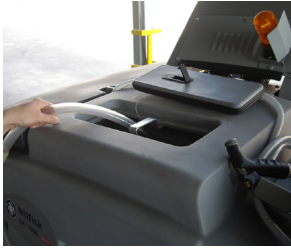
2. Fill the tank with clean water. The clean water temperature must not exceed 40 °C
