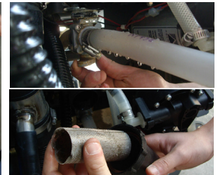
15. Close the solution tank valve and remove and clean the filter
