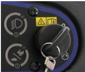
7. Turn the ignition key to "I" and press the throttle button (if you want to raise your rpm from idle)
