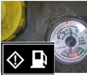
1. Check the Diesel fuel tank level / LPG bottle charge. In case re-fill/ change the LPG Bottle
