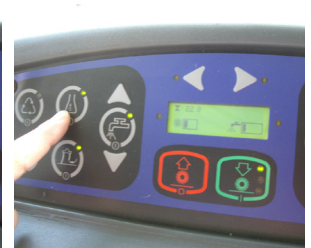
10. Adjust to the desired chemical concentration (shown in the display)
