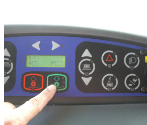
8. Lower the deck and select the desired scrubbing pressure (squeegee lowers automatically)
