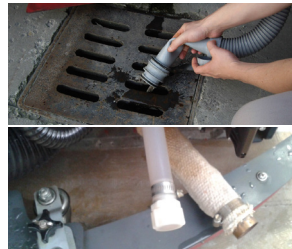
13. Empty the recovery tank with the hose. Then empty the solution tank with the transparent hose
