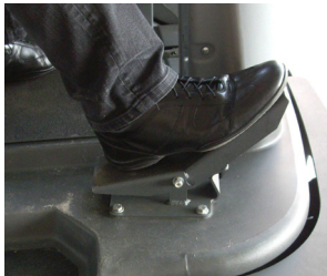
11. Press the forward pedal and start operating the machine – all functions will activate upon the motion of the pedal
