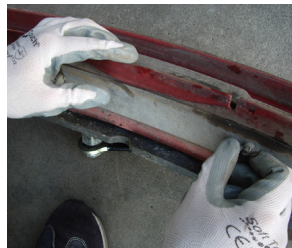
18. Take the squeegee off, check the blades wear status
