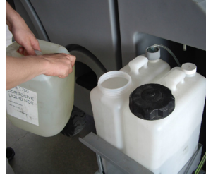
3. Fill the Ecoflex tank with a detergent suitable for the work to be performed (highly concentrated detergent)
