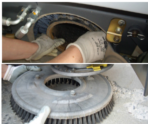
6. Install the cylindrical broom/side brush or brooms
