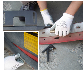
19. Remove the side skirts and check the blade status
