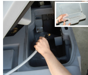
14. Wash with clean water the recovery tank and the vacuum grid. Remove and clean the debris tray
