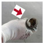
If necessary open the solution filter cage and clean the net
