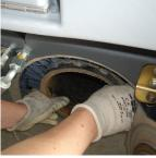
Open broom door compartment and check presence of roped or debris that can block it
