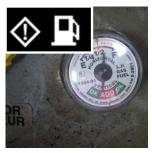
1 Check the Diesel fuel tank level / LPG bottle charge. In case re-fill/ change the LPG Bottle
