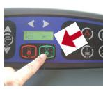
2 Make sure that deck and squeegee 3 Adjust the water flow are moving down when pressing the button
