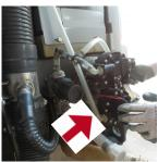
Solution valve must be open and solution flow pump hoses filled
