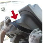
3 Recovery tank seal cover must correctly installed and in good
