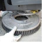
Remove and clean the brushes. Check they rotates and touch the floor properly
