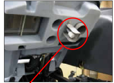
Recovery Tank Full Switch S2
