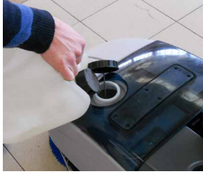
2. Fill the tank with a solution suitable for the work to be performed.
