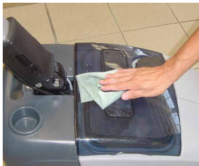
16. Clean the machine using a damp cloth and where needed use a neutral cleaning product.
