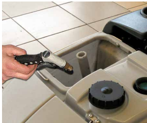
11. Wash with clean water the recovery tank.
