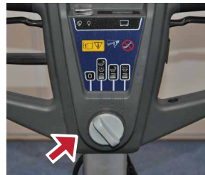
9. Turn the knob to "0" position to switch off the machine.
