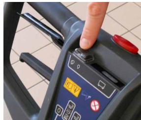
7. Press the solution flow control switches as necessary, depending on the type of cleaning to be performed.
