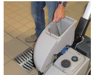
10. At the end of the work. Empty the recovery. Then empty the solution tank.
