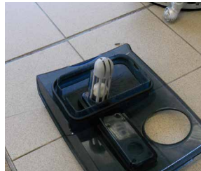
12. Wash with clean water the vacuum grid.
