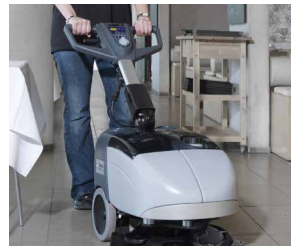
8. Press the enabling push-button together with the brush levers for starting floor cleaning. If solution applied flows outside the brush housing during use, reduce the flow of solution.
