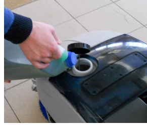
3. Always follow the dilution instructions on the label of the chemical product used to prepare the solution. The solution temperature must not exceed 40°C and be none foaming
