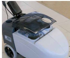
18. Park the machine with the recovery tank cover open.
