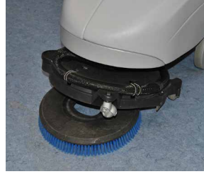
4. Place the brushes or the pad-holders under the deck. Use the appropriate brushes to clean the floor.
