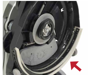
14. Take the squeegee off and remove debris.
