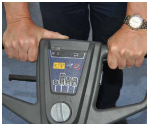
6. Press the enabling push-button together with the brush levers to engage the brush/pad-holder and then release it.
