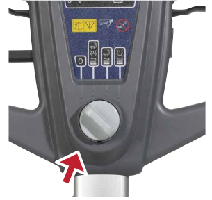
4 Check if the programs selector is damaged or has the right function selected.
