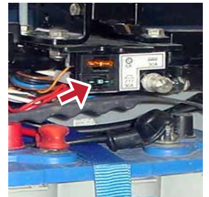
4 Check if the fuse isn't burnt out.
