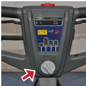
1 Check if the programs selector has the right function selected.
