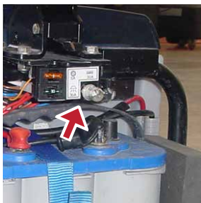
1 Check if the fuse has triggered.
