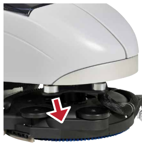
2 Check if there are external materials avoiding brush rotating.
