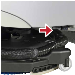
1 Check if the suction hose is correctly installed and cleaned.
