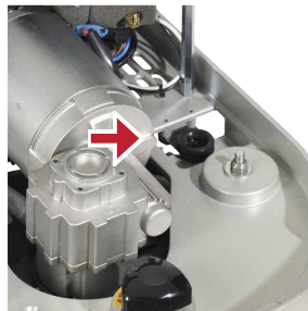
2 Check if the solution valve is dirty/clogged.
