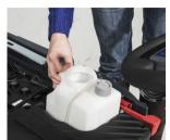
3. Fill the  $\mathsf{EcoFlex}^\mathsf{TM}$  tank with a detergent suitable for cleaning machines (highly concentrated and low foaming detergent).
