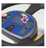
Check if the green switch Led of the One-Touch button is flashing. Wait until the light is steady.
