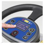
1 Check if there isn't any brush motor 2 Check if the brush are correctly overload "WARNING ALARM F2" on the display.
