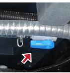
2 Check if the solution valve is open. 3 Check if the solution filter is
