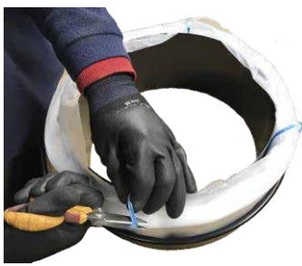
5- Cut and remove the LONGOPAC® closing bands.
