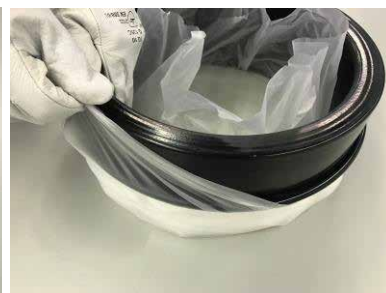
7- Pull the outer part of the bag to create the new one.
