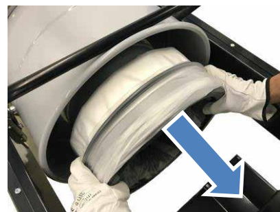
3- Remove the LONGOPAC® container and any waste.
