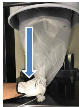
3- Pull the LONGOPAC® end to make a new bag.
