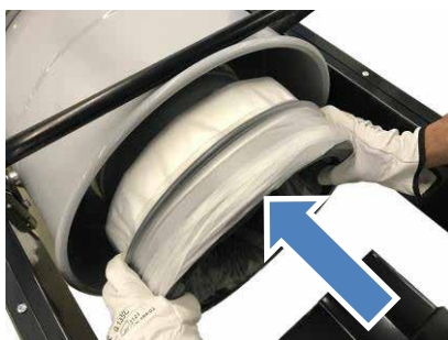
8- Insert the container with the LONGOPAC®.
