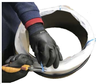
5- Cut and remove the LONGOPAC® closing bands.
