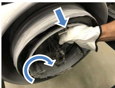
2- Pull and rotate the retaining pins of the LONGOPAC® container in order to unfasten them.
