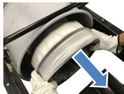
3- Remove the LONGOPAC® container and any waste.
