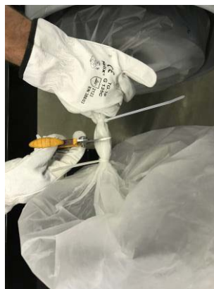
2- Cut the strip between the two bands.
