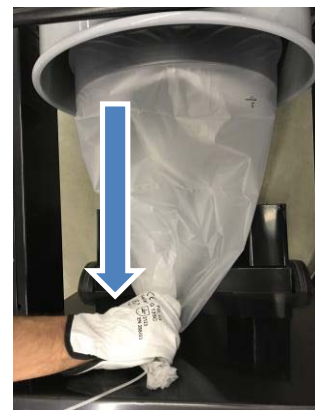
3- Pull the LONGOPAC® end to make a new bag.
