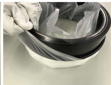
7- Pull the outer part of the bag to create the new one.
