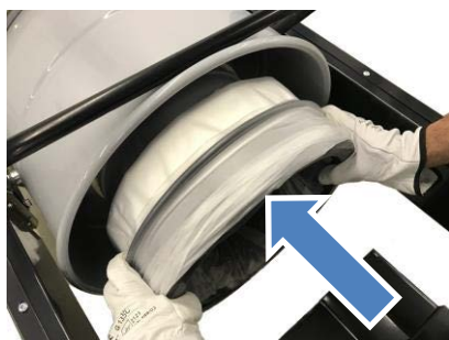
8- Insert the container with the LONGOPAC®.
