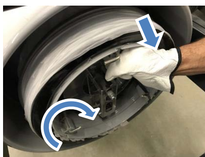
9- Pull and rotate the retaining pins and insert them into their seats.
