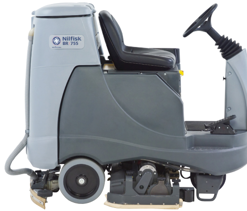
↑ Front and rear polyurethane wheels for outstanding traction and high durability
