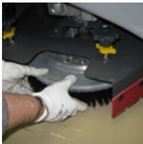
1 Check if the brush are correctly installed and not worn out.
