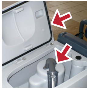
2 Open the recovery tank and check if the vacuum grid and gasket are cleaned.
