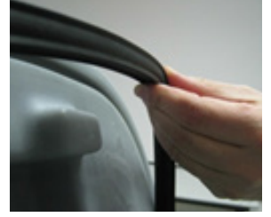
4 Recovery tank seal cover must correctly installed and in good condition.
