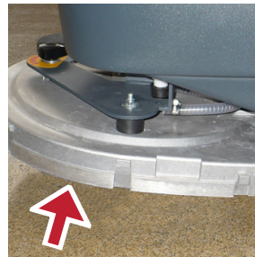
3 Check if there are external materials avoiding brush rotating.
