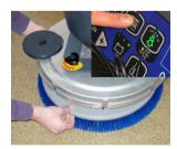
15. Press the switch and wait for the brush to fall on the floor. Remove the brush and clean them.
