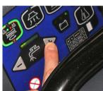
7. Press the solution flow control switches as necessary, depending on the type of cleaning to be per formed.
