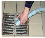
12. At the end of the work. Empty the recovery tank with the hose. Then empty the solution tank with the trasparent hose
