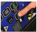
8. Press the detergent flow control switch. The number of display shows the detergent concentration level in the ing power. solution (see the table on the label). See the User Manual for setting change
