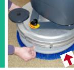
1. Check if the brush are correctly installed and not worn out.
