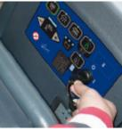
3 Turn the ignition key to "0", then try to start the machine without pressing the paddle.
